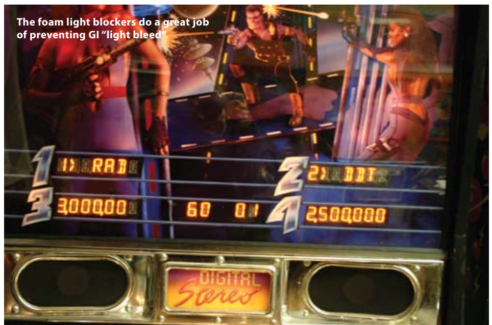
The replacement PinScore displays, installed and working
