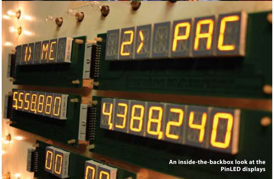
The PinLED Displays, Installed and working
